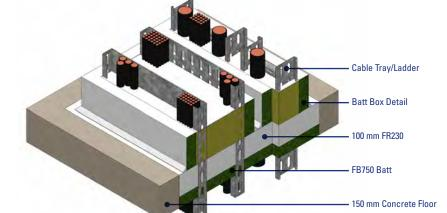
Cables penetrating through a rigid floor construction. 100 mm of FR230 installed onto a 50 mm 140 kg rock fibre shutter batt to form a 150 mm overall seal depth. A 'batt box' 150 mm deep is installed on top of the FR230 seal, comprising a lining 150 mm thick FB750 infilled
